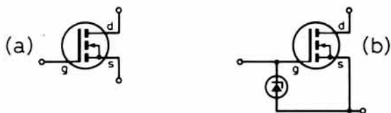
Fig 1. (a) Schematic symbol of the standard unprotected vmos device. (b) The protective gate diode found in many switching devices
