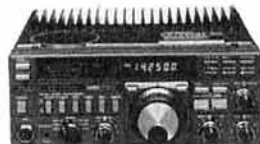
IC 271 — Icom's v.h.f. multimode base station
